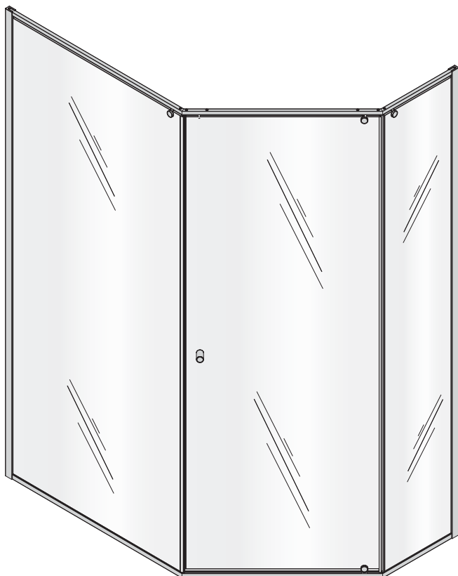
MOQP 1200 X 900 LH CORNER (OFFSET) CAN HINGE FROM LEFT OR RIGHT
