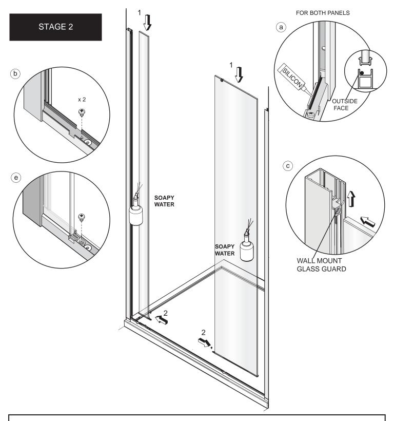
This stage is describing the fitting of both fixed panels. Before fitting the fixed glass panels adjust the threshold extrusion so that it is equally positioned between the two wall mounts. Loosen the threshold adjusters at each end and lightly tighten in position as required.
