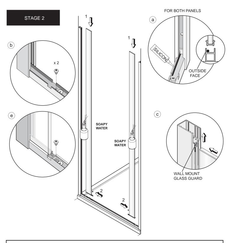
This stage is describing the fitting of the both fixed panels. Before fitting the fixed glass panels adjust the threshold extrusion so that it is equally positioned between the two wall mounts. Loosen the threshold adjusters at each end and lightly tighten in position as required.
