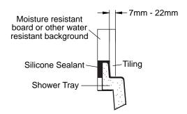
Alternatively, bottom of wall may be cut back to allow tiling lip to be flush with wall.
