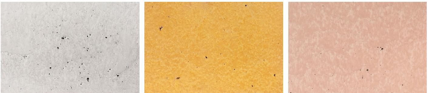
Due to the nature of the casting process, air trapped within the concrete can sometimes cause small holes to form within the surface. These can vary in size and add to the distinctive texture and aesthetic of concrete.
