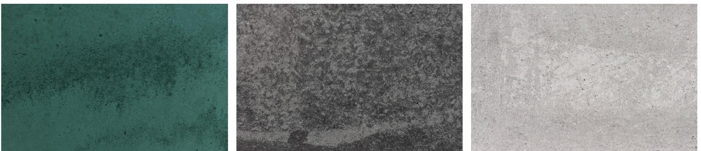
Concrete will never be a monotone block colour due to the number of variable materials from which it is made. The variations in tone and texture create a unique patina that is integral to the character of concrete.
