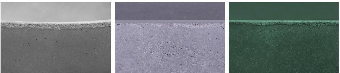
Some basins require two-part moulds which can result in a different texture around the edge where the two moulds meet. This is where moisture within the mix can evaporate out at the seam creating a more raw, distinguished texture.
