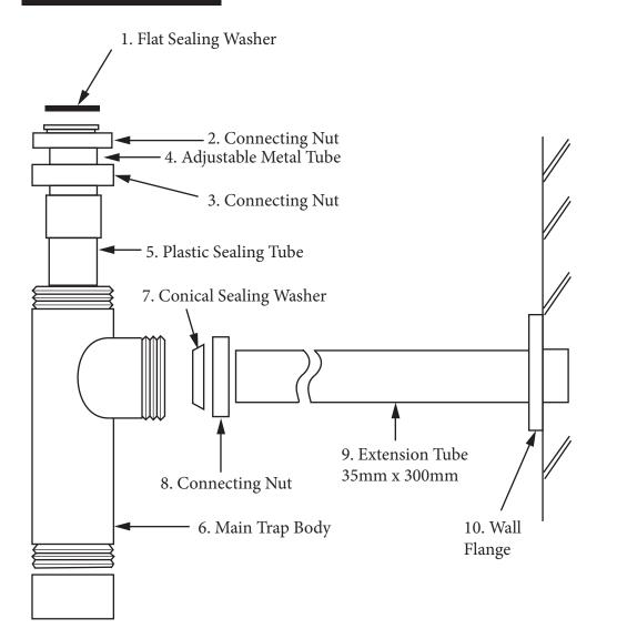
This bottle trap is supplied fully assembled, check all components shown on the drawing are present.
